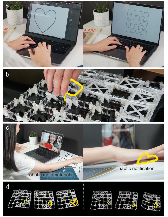
Figure 20: (a) A user designs a heart path for their haptic notification, and receives cell configuration from our software. (b) They insert cells as shown in the software. (c) When video-chatting with a friend, Robotic Metamaterials integrated into their desk renders a heart shape on their palm. (d) The same Robotic Metamaterials configuration is able to draw other symbols, such as a water drop.
