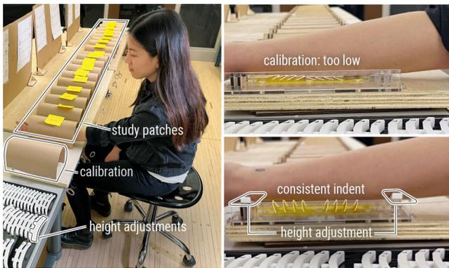
**Figure 9: Study setup.** Before conducting the study, each participant’s arm is first calibrated for consistent indentation of the tactors into the skin.
