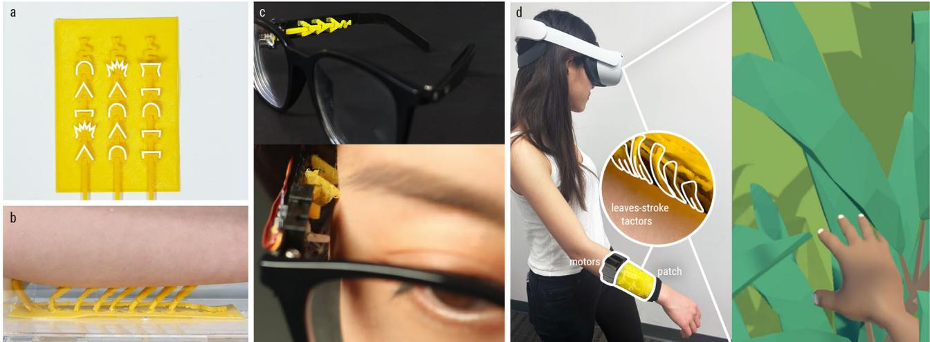
**Figure 1:** We present customizable and versatile haptic patches that are lightweight, reconfigurable, and can be integrated as wearables or into objects. (a) Users can customize their own haptic patches with a software design tool we provide. (b) One linear pull can actuate many factors, producing haptic sensations on a large area of the skin. Our approach can, e. g., be integrated (c) into existing worn objects, or (d) designed for VR experiences.
