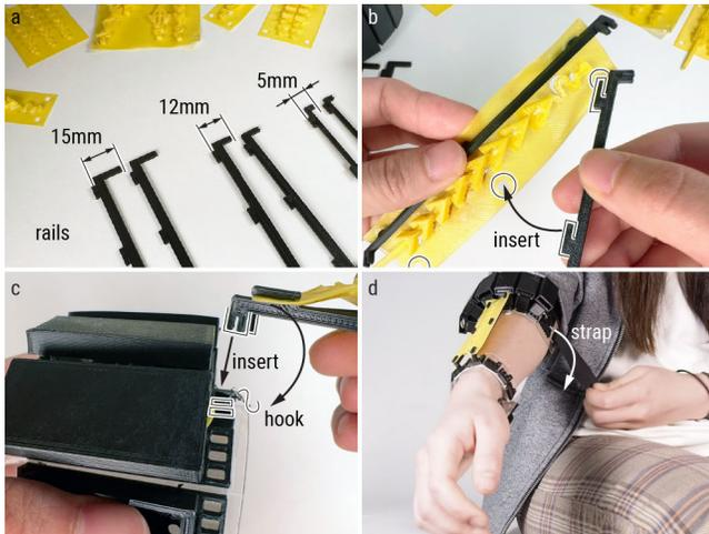
**Figure 5:** (a) Rails of various heights accompany varying tactors. To put a haptic patch onto the wearable, (b) users would insert a pair of rails into slots on the patch, (c) and insert these rails into slots on the wearable. The tactors are connected to the motors by hooking pull strings (i. e., end of a stem structure) to the motor mounts. (d) users can wear the motor-actuated haptic patch using straps on the wearable.
