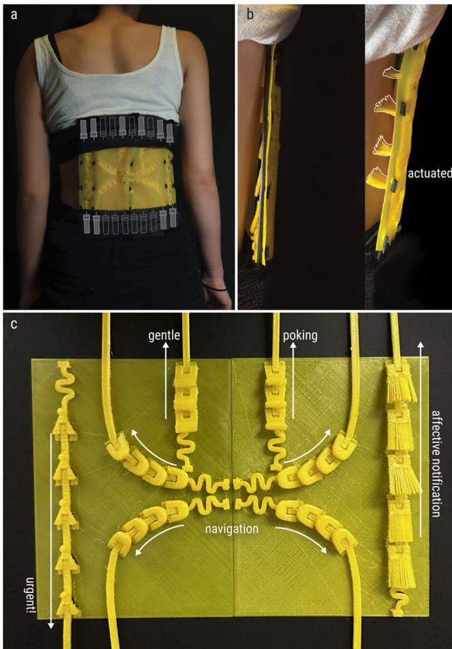
**Figure 13:** (a) This back wearable patch delivers various notifications and information to the user’s lower back. (b) The user gets a gentle notification for a text message from their family. (c) We show the various tactors and directions we can render on this larger area.
