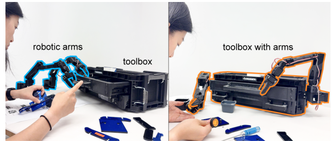
Fig. 1. We augment task-centric objects, such as a toolbox, with robotic arms to become object-embodied collaborators.
