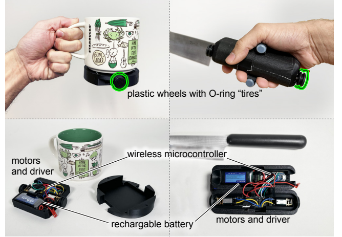
Figure 6: We augment everyday objects, such as coffee mugs and kitchen knives, with small wheels that allow them to move across flat surfaces. These robotic objects are controlled wirelessly by our motion subsystem.
