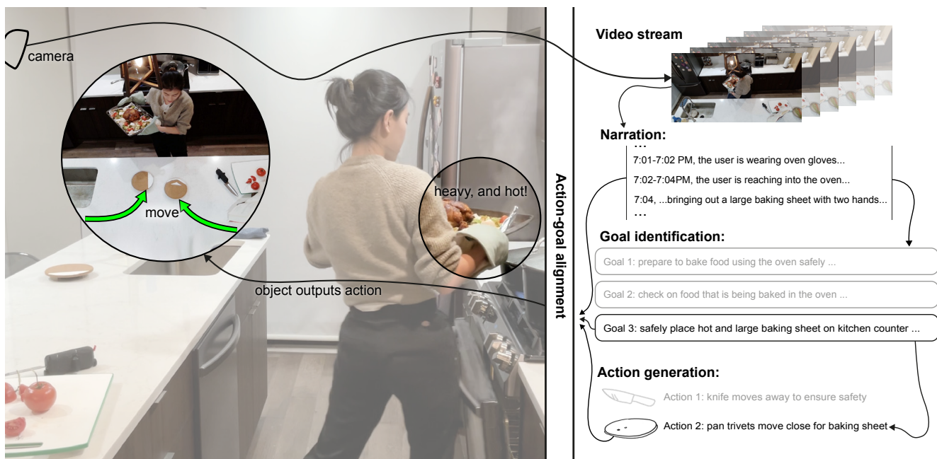
Figure 1: Everyday objects, such as trivets, are brought to life by the Object Agents system. These objects move autonomously, in order to assist and protect users. Our system (1) perceives context using a vision language model backbone, (2) reasons about user goals and object affordances, and (3) generates actions that are delivered to familiar items augmented with robotic motion.
