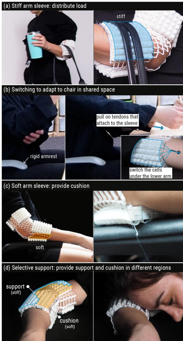
**Figure 10:** Our arm-worn material interface (a) can provide a protection padding when holding a bag during traveling, and (b) allow users to adjust the stiffness to adapt to the chair in shared spaces, (c) to have a more cushioned arm-rest. Users can use the upper part as (d) a selective-support cushion for a power nap.
