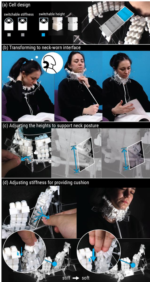
**Figure 14:** (a) Our collar is designed with columns arranged around the neck, each column consisting of three types of cells. (b) The collar can be transformed into a neck support when the user feels strain in the neck. (c) Users can adjust the height to fine-tune their neck posture. (d) Additionally, users can modify the local stiffness for comfort.
