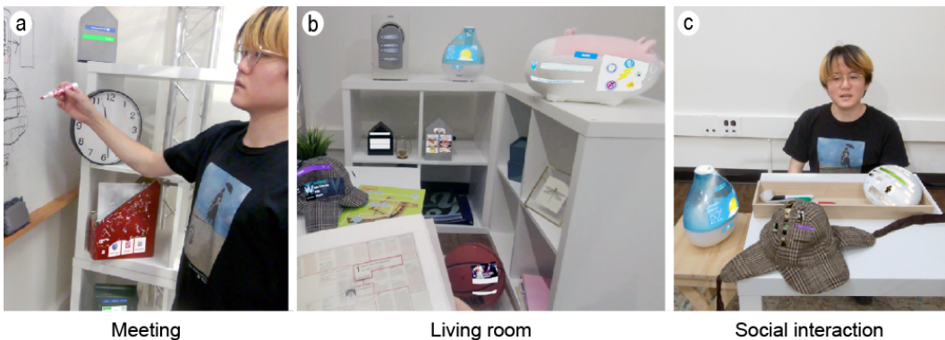
Fig. 11. Implemented application scenarios. (a) In the meeting scenario, the red folder and gray decorative object hold virtual objects. (b) In the living room, weather applications and quick access for other apps are visible. (c) Similar pairings between 2D applications and physical objects are shown in the social interaction scenario. All images were recorded live through the Varjo XR-3 MR headset.
