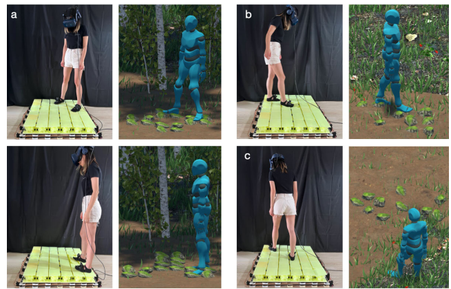
Figure 18: We can (a) reconfigure our interactive floor’s stiffness dynamically, (b) activate pre-programmed patterns (e.g., stepping stone), or (c) make the entire floor rigid or soft.
