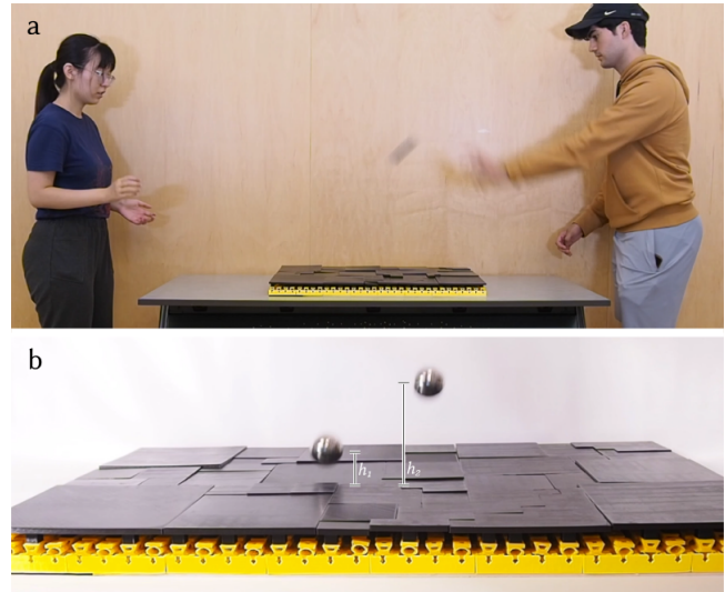
Figure 12: A ball game that combines pong and battleship. (a) Users throw a ball onto the material, but could previously configure (b) the local elasticity to make it difficult for their opponent to catch the ball. The map is concealed as the configuration layer looks identical from the top.
