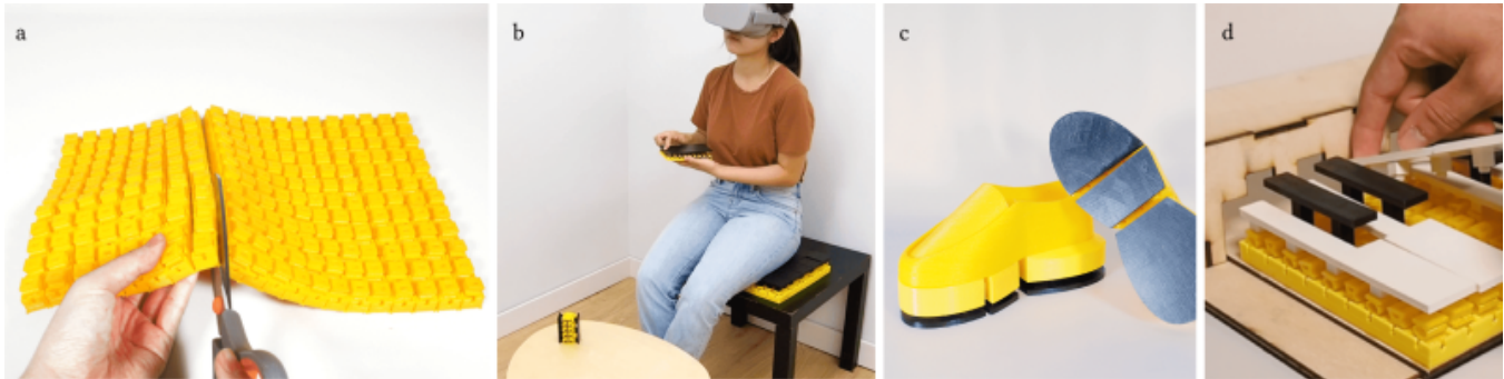
Figure 1: We propose a reconfigurable metamaterial that can be easily and repeatedly reconfigured by end users. We envision (a) that the generic material sheet can be purchased as larger sheets, and be cut and configured to opportunistically augment the elastic properties of objects. We show how this material can be applied to realize applications, such as (b) passive haptic props for VR, (c) custom shoe soles or (d) piano keys.
